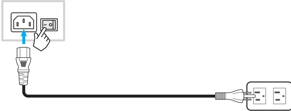
Press the **Power** button to turn on the IFP. The LED indicator light turns blue, indicating it is ready to use.
